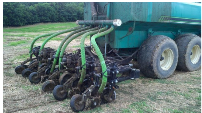
Figure 2. Manure injection unit with six injectors spaced 30 inches apart.
