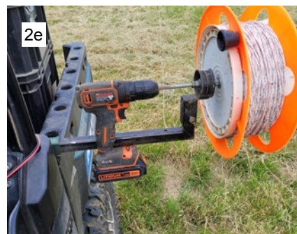
2e. A standard extension cord reel adapted for use with a battery-powered drill eliminates the need to reel up poly wire by hand.
