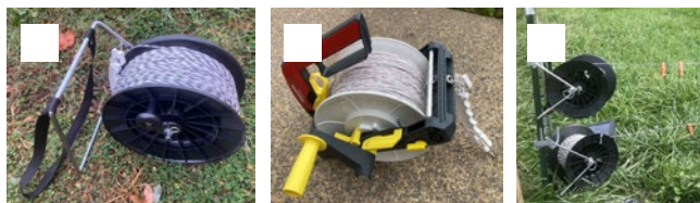
Figure 8. Examples of a nong geared reel with strap (a), a 3:1 geared reel (b), and a post with reel holders (c).
