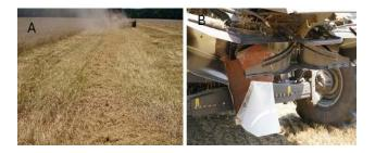
Figure 3. A) Weed seeds and chaff narrowed down into a line during wheat harvest, B) Chaff liner fixed behind the harvester to concentrate chaff and weed seeds therein.
