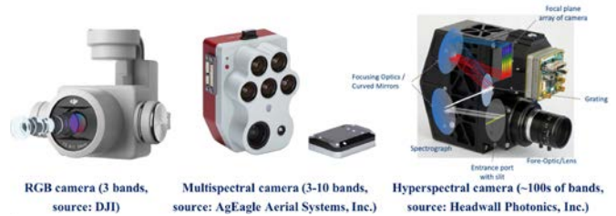
Figure 1. Examples of market-available drone mountable RGB, Multispectral, and Hyperspectral cameras.
