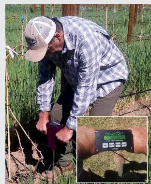
Figure 12. Penetrometer being used to measure soil compaction in a young vineyard. Inset is digital readout of resistance in pounds per square inch (PSI). In this example, 165 PSI equates to 1.14 MPa. (Photos courtesy of Gill Giese, New Mexico State University.)
