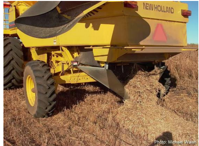
Figure 4. Example of combine modifications for narrow windrow burning. (Photo by Michael Walsh.)
