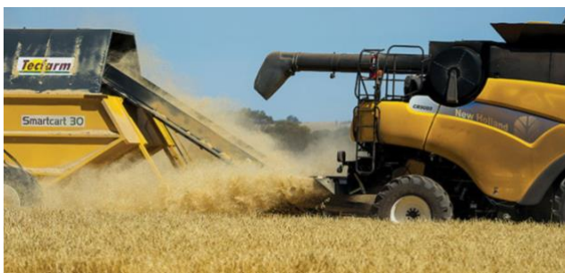
Figure 4. Example of a chaff cart system. Photo: Evan Collins.
