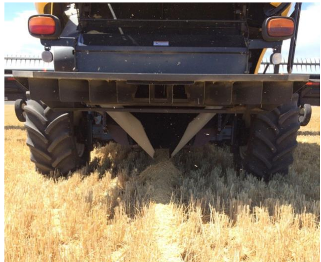
Figure 5. Example of combine modifications for chaff lining. (Photo by WeedSmart.)
