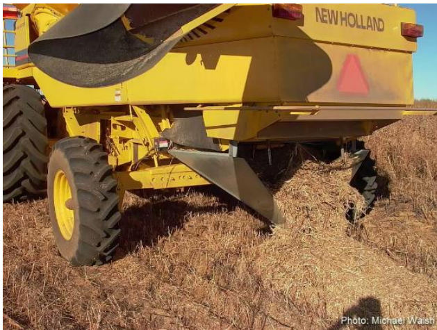
Figure 3. Example of combine modifications for narrow windrow burning. (Photo by Michael Walsh.)
