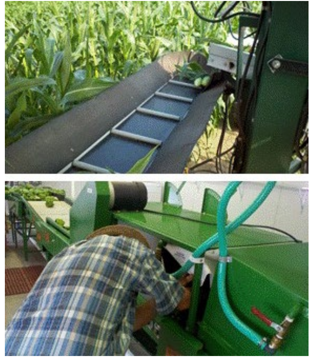
Figure 6. Harvest equipment, like this conveyer system used for sweet corn that has been hand harvested, is kept properly cleaned and maintained (top). A grower collects a sample of packing line spray water to make sure the chlorine sanitizer concentration that is being sprayed on to the green peppers meets pre-determined chlorine levels (in parts per million) (bottom). (Vallotton)
