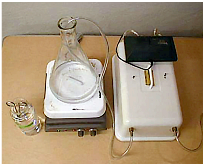
Figure 2. Example of a lab-based ozone generator. (Photo courtesy of Rob Williams, Food Science and Technology, Virginia Tech.)
