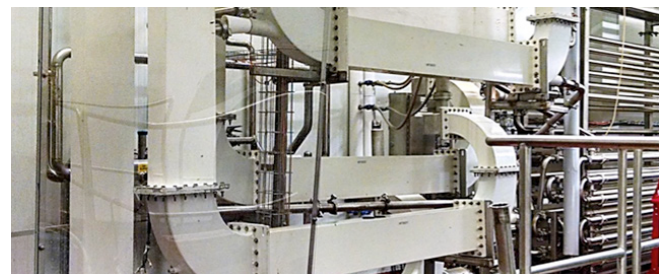
Figure 2. A commercial microwave processing system developed by the food engineering team at North Carolina State University. (Photo courtesy of Josip Simunovic, Department of Food, Bioprocessing and Nutrition Sciences, NC State University.)
