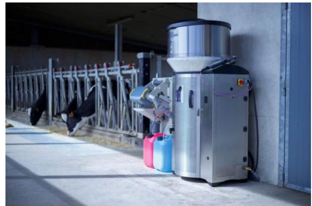
Figure 2. An automated combi feeder installed by a calf pen.
