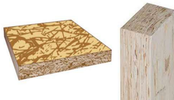
Figure 3: Laminated Strand Lumber (LSL).(CWC, 2021b; Naturally Wood, 2021a)
