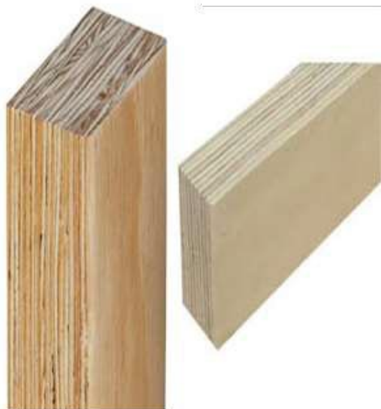
Figure 2: Laminated Veneer Lumber (LVL)(Chirag Enterprises, 2021; CWC, 2021a)
