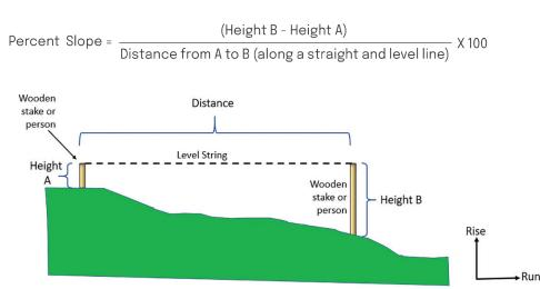
**Figure 4:** Determining slope in the field. Note that a small string level can be used to ensure that the string is level (or you can eyeball it).
