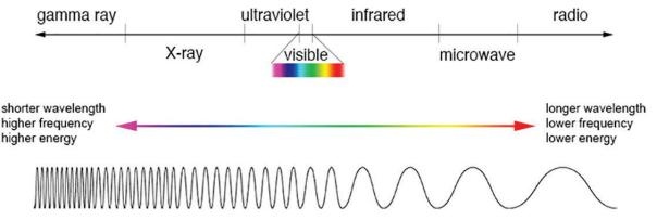
Figure 27: The visible and invisible range of the electromagnetic spectrum.
