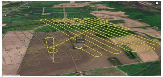
**Figure 29:** Example of an oblique perspective of a digital flight plan.
