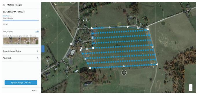
Figure 41: The Upload Images screen on DroneDeploy. Each blue dot represents an image that is being uploaded.
