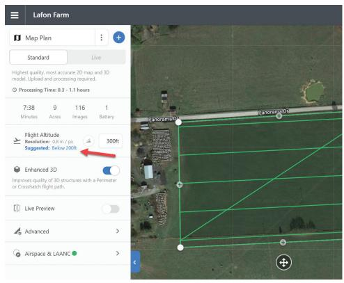
Figure 34: Autonomous Flight Planning in DroneDeploy.
