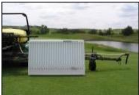
Figure 16. Check spray pattern uniformity.
