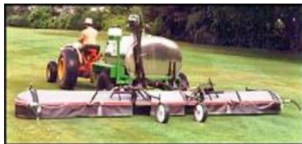
Figure 11. Shield booms minimize the effect of wind on the spray pattern and thereby reduce drift potential.
