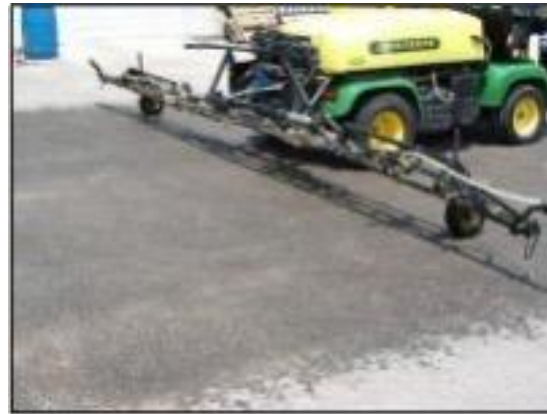
Figure 19. Check spray pattern uniformity by driving over a hot pad of road surface and watching the drying pattern.
