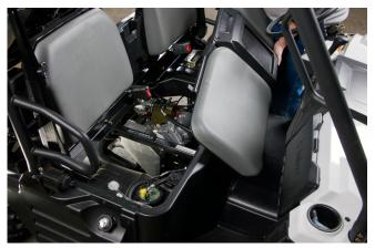
Liquid-cooled engine with radiator under the seat.
