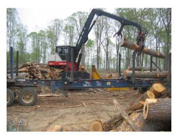
A log deck is an area of high activity and high impact where logs are concentrated, sorted, and loaded onto trucks.
