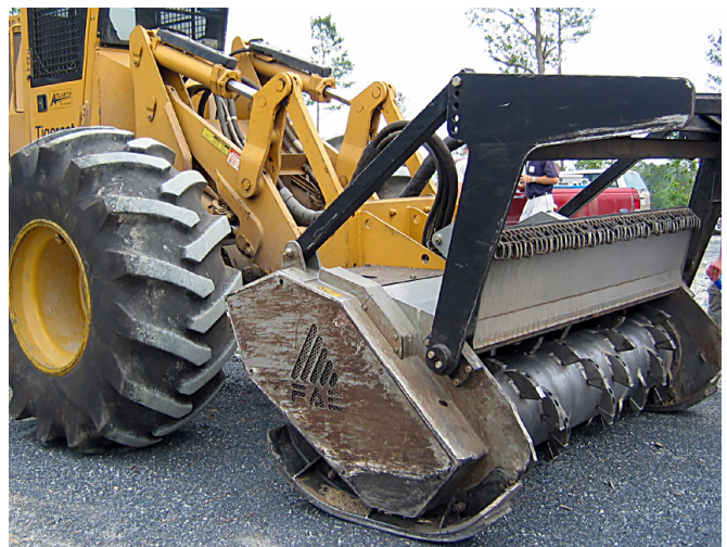
Figure 1: Large rotary mulcher. Photograph by Adam Downing
