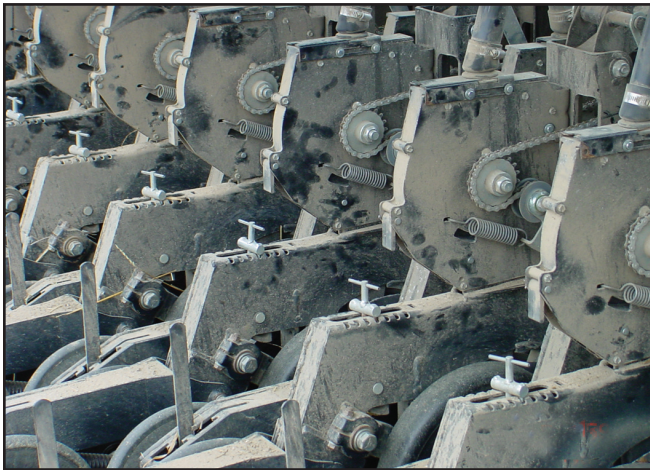
Figure 3. Seed metering for seed singulation on a grain drill. Meter device is shown with gear and chain drive. (see figure 4 for location)
