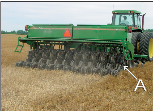
Figure 4. Precision seeding system with seed meters close to the ground. a) marks the metering device.
