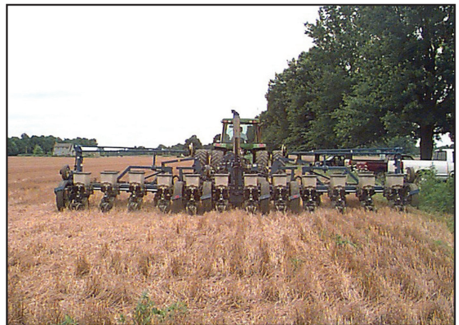
Figure 5. Planter equipped with extra planter boxes to plant 15-inch rows.
