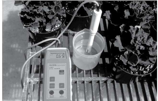
Figure 2. Portable electrical conductivity (EC) meters can be used to measure the EC of the dilute fertilizer solution to verify that the injector is working within the expected range. Compare the EC of the solution to that recommended on the fertilizer bag (Fig. 3) or the fertilizer label.
