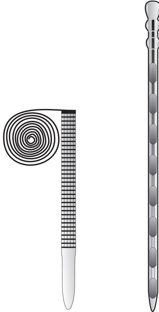
Figure 3. Probe Trap      Figure 4. Grain Trier
