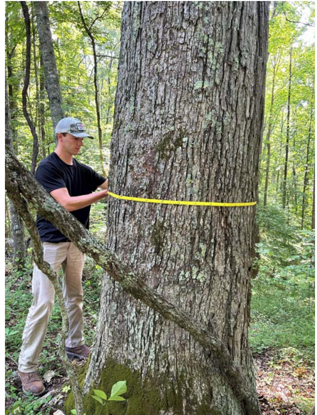
Figure 1. Forester measuring the diameter of a white oak tree using a diameter tape held at breast height, or 4 1/2 feet from the ground (Photo by Bill Worrell).
