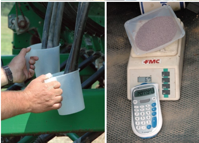
Figure 6. During stationary calibration, the drive wheel is turned and the seed is caught and weighed.
