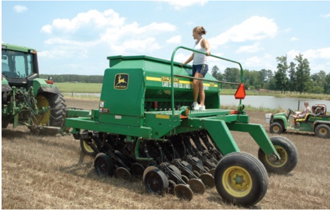
Figure 2. No-till grain drills are commonly used to establish small-seeded forages. They consist of a no-till coultter (some drills) that cuts a slit into the soil, followed by disc opener that places the seed in the soil, and a press wheel that establishes good soil-to-seed contact.
