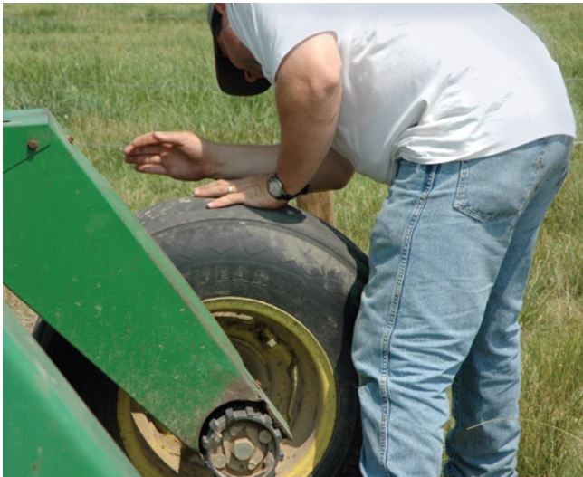
Figure 5. The drive wheel on a grain drill can be jacked up off the ground and turned a given number of times to obtain the desired coverage area.
