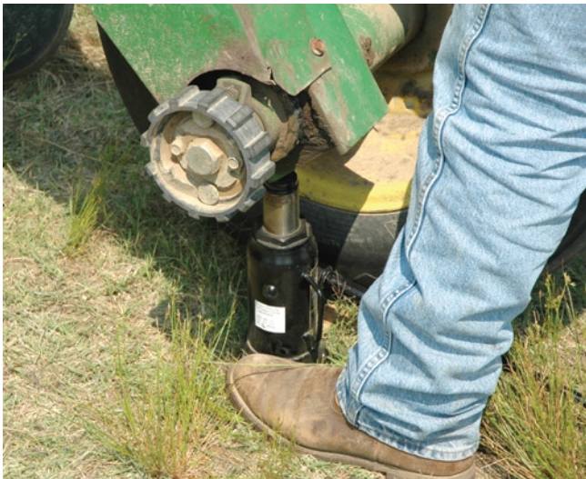
Figure 5. The drive wheel on a grain drill can be jacked up off the ground and turned a given number of times to obtain the desired coverage area.
