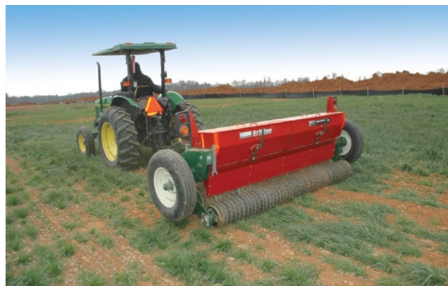
Figure 1. A cultipack seeder is a type of drop seeder that consists of two offset corrugated rollers with a metering box between them. The first roller firms the soil, the seed is dropped between the rollers by the metering box, and the second roller presses the seed in contact with the soil.
