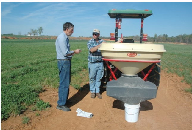
Figure 3. A spinner- or pendulum-type spreader can be used to broadcast seed. The pendulum spreader above is equipped with a special attachment that allows broadcast seed to be collected in a bucket and weighed during calibration.
