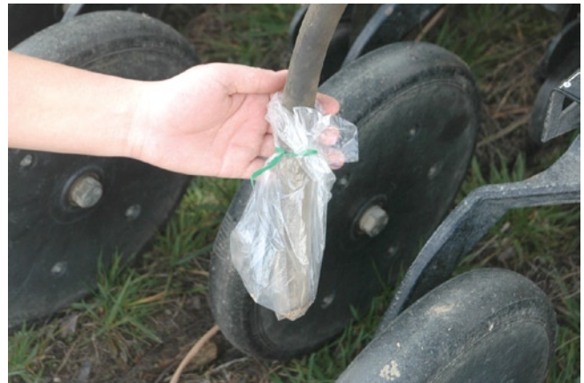
Figure 4. Seed tubes on a grain drill can be disconnected and a plastic bag placed on the seed tube to collect the seed during calibration.
