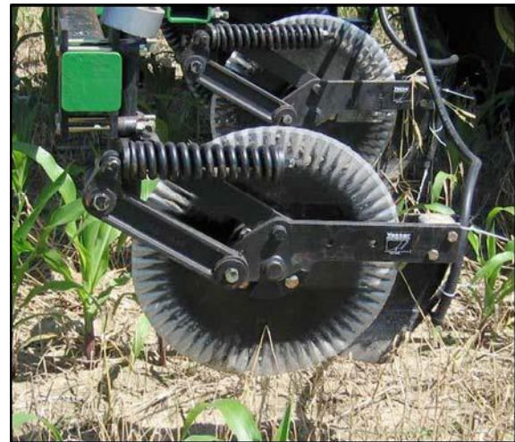
Figure 1. No-till opening coulters
