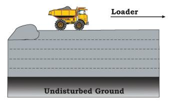
**Figure 3.** A representation of mine-spoil pad construction using loaded haul trucks to achieve compaction. In order for this procedure to be effective, truck traffic must achieve compaction over the entire building-support pad area, while lift thickness and spoil composition must be tightly controlled. In an ideal situation, specialized compaction equipment would be used on each lift.
