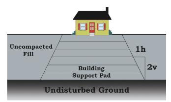
**Figure 2.** A representation of a mine-spoil pad constructed to support an intended building site during reclamation. The spoil pad should extend beyond the minimum area required to support the building. In most cases, the zone where the surface is compacted should extend at least 10 feet beyond the intended footing area. The compacted spoil pad should extend downward at a minimum angle of about 30 degrees from the vertical (a 2v:1h slope).
