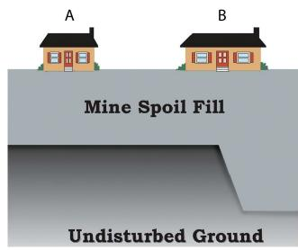
**Figure 1.** Settlement of underlying mine spoils can affect buildings constructed on mine-spoil fills. The spoil depth under building A (left) is relatively uniform, whereas building B (right) is built over an area where spoil depth varies. Building B is more likely to be damaged by differential settlement because it covers a larger lateral area and because of variations in the depth of the underlying spoils.
