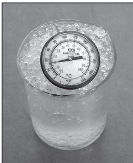
Figure 1b: Correctly calibrated thermometer in a mix of crushed ice and water.
