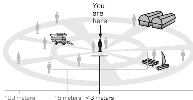
This reporting information is particularly important when comparing GPS receivers. A 2DRMS accuracy specification is twice as big as the RMS specification for the same unit. The RMS specification is about 1.2 times the CEP accuracy. Therefore, a unit with “5-ft 2DRMS accuracy” is actually more accurate than a unit with “3-ft RMS accuracy” since “3-ft RMS” is equal to “6-ft 2DRMS.”
