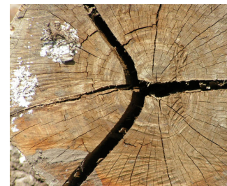
Figure 1. A log with extensive mechanical and biological damage due to improper inventory handling conditions.
