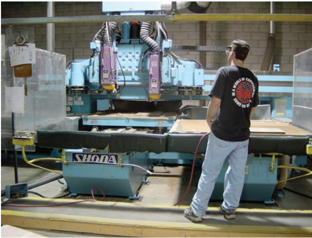
Figure 7. Computer numerical control (CNC) equipment with dual table used in an institutional furniture factory.
