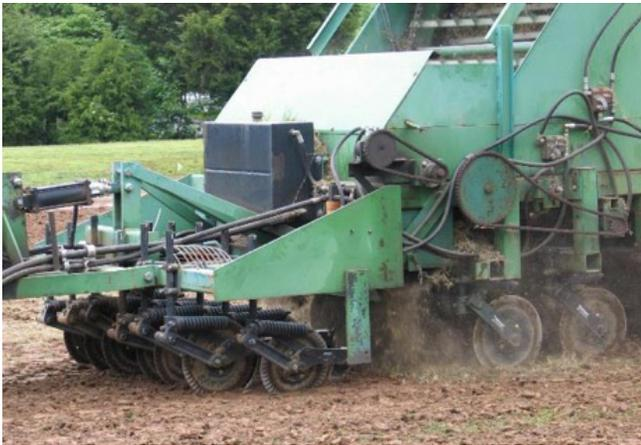
Figure 9. Shredded stems (sprigs) of creeping grasses like bermudagrass and zoysiagrass can be used as another means of vegetative establishment called “sprigging,” where the stems are pressed into the ground of a prepared planting bed. (Photo by author.)
