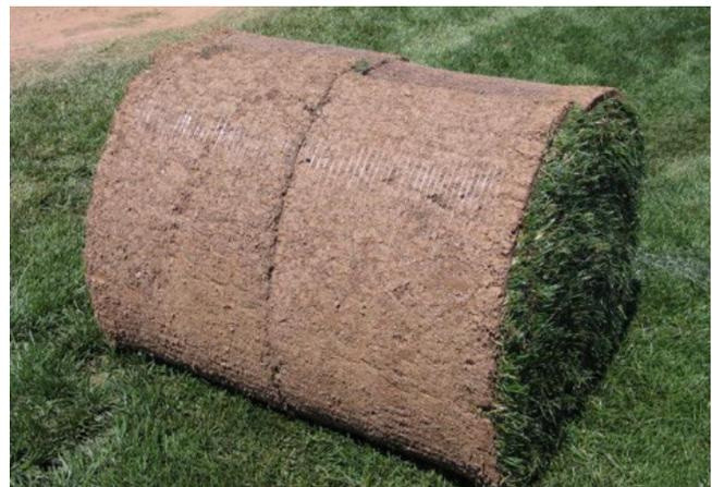
Figure 7. This sod was netted at harvest in order to improve its handling characteristics. Be sure to find out whether or not a sod is netted in order to best meet project needs. (Photo by author.)
