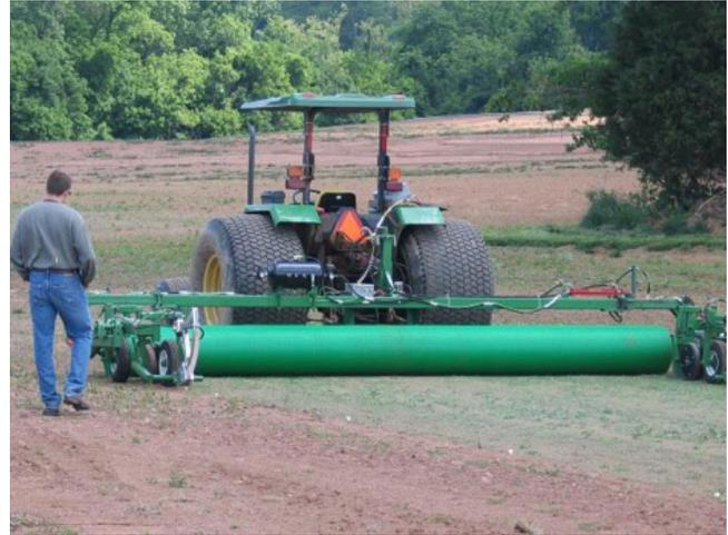
Figure 6. Polypropylene netting is often installed in the field after seeding to improve the tensile strength and the rate of harvest of the pending sod crop. (Photo by author.)
